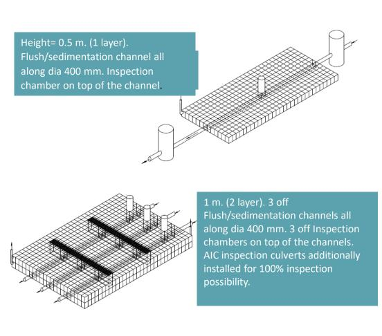
3 off Inspection chambers on top of the channels. AIC inspection culverts additionally installed for 100% inspection possibility
