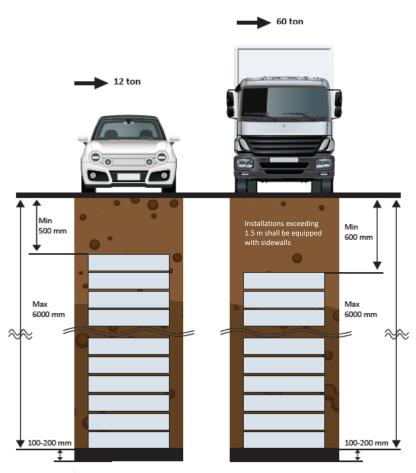
At Installation in green area we recommend min cover of 450 mm.
